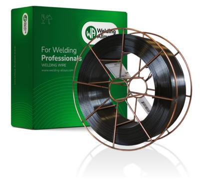
HARDFACE HC-O is a self shielded flux cored wire with a high chromium cast iron deposit, containing a high proportion of hard primary chromium carbides in a tough austenitic matrix.
